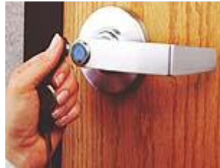
Figure 4: how java ring is used to open the door
