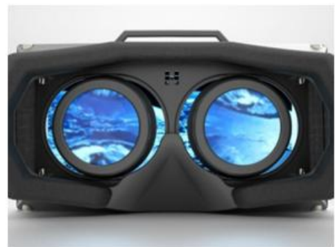
Figure 3: The Rift with its immersion-producing lenses
