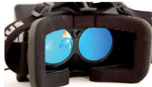
Figure 2: The Rift with its immersion-producing lenses
