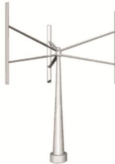
Figure 2.2. An H rotor VAWT .
