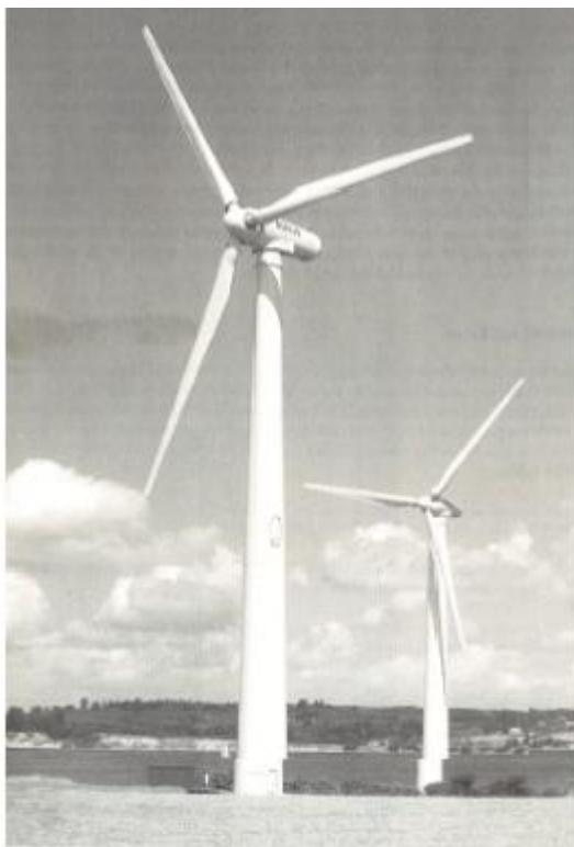
Figure 2.3. A 450 kw HAWT with 37 m rotor diameter (Bonus).
