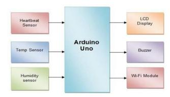
In this paper we are going to build a RHM(Remote Patient Health Monitoring System)using IOMT. Firstly we will attach the sensors to the patients body namely
